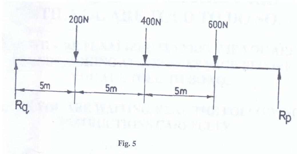
A simply supported beam of span 20 metres carries three vertical load as shown in Fig. 5.
