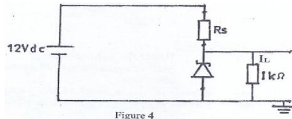
In Figure 4, a 5 V stabilised power supply is required from a 12 V d.c. input source. If the maximum power rating of the zener diode is 2 W, calculate the
